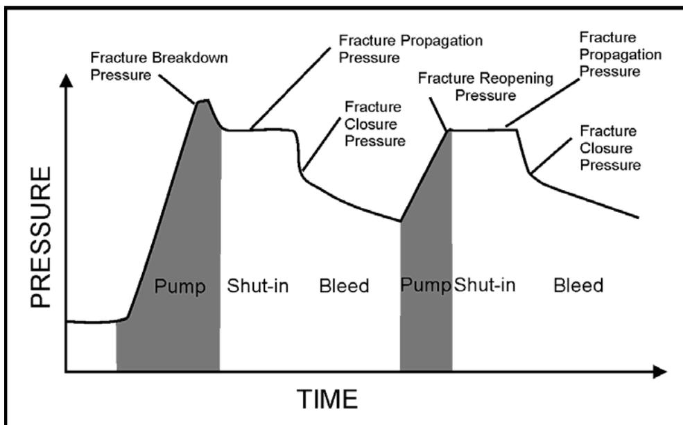
**Figure 1. Simplified pressure-time chart characteristic of a hydraulic test [Bell, 1996 (cited in Horwarth and Wille, 2009)]**
