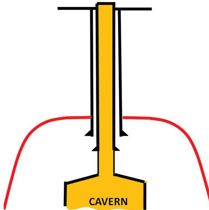
**Figure 3. Two cemented casings anchored to the salt formation**
