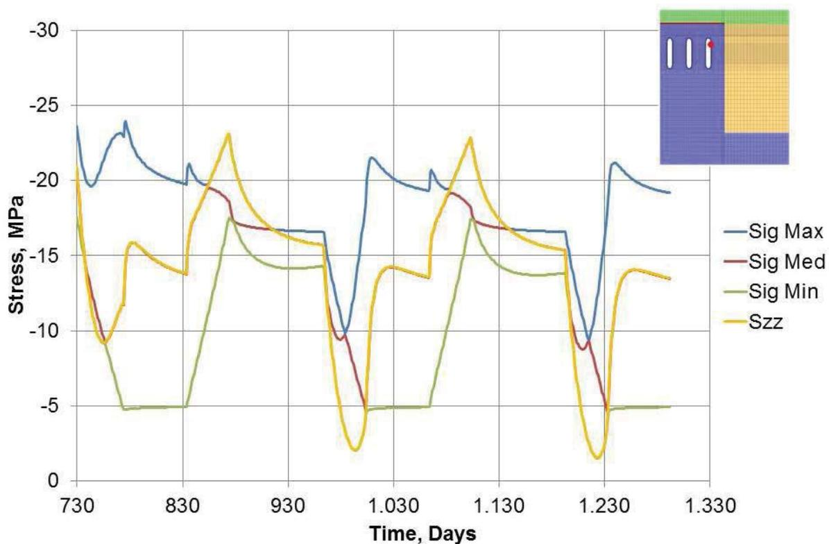
**Figure 5. “Principal Stress Components at the Assessment Point in the Roof Section of the Border” (Zapf, 2014).**
