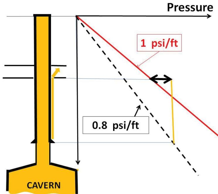
**Figure 2. Illustration of a gas leak: the vertical pressure gradient is 1psi/ft, and the maximum pressure gradient is 0.8 psi/ft**
