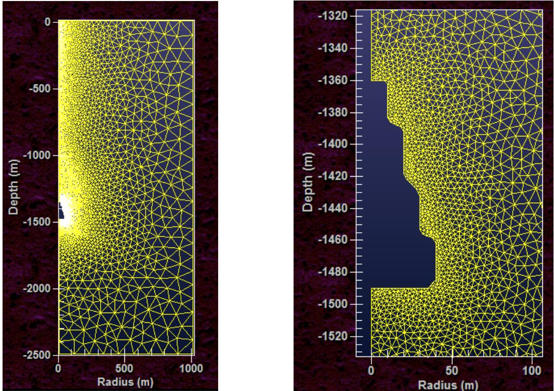
Figure 5 - Rock mass mesh (left) and mesh in the cavern area (right).
