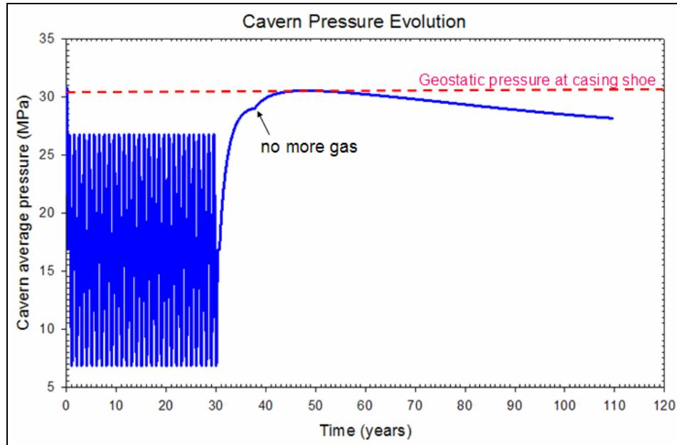
Figure 10 – Cavern pressure evolution, Case 5 — 6-month waiting period,  $V_g = 300 \text{ m}^3$ , small leak.
