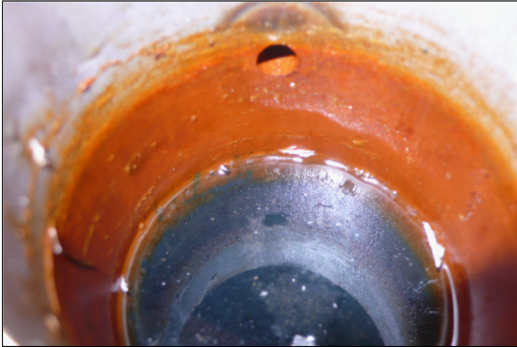
Photo 3 – The hole above the 7" string that allows brine evacuation.
