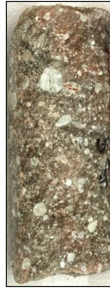
Figure 18 – Core-sample from SPR3 at a depth of 713 m. (Inclusions total about 15%.)
